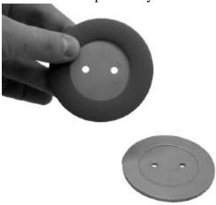
NOTE: Apply Loctite 271 (or equivalent) to the screw threads. Be sure the cup is evenly spaced on the plunger disc and support.
