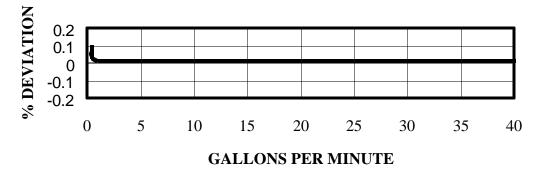
The 682 meter's linear accuracy (percent of error over or under the zero - error level) remains within design parameters (+/- 0.2%) over its 0.2 to 40 GPM flow range. This exceeds the maintenance requirements for accurate custody transfer of product, as specified in the National Institute of Standards and Technology (NIST) Handbook 44.
