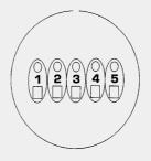
Hall Effect Voltage 4.5 to 24 VDC Current Draw Minimum 4.6mA Output NPN Open Collector 25mA
