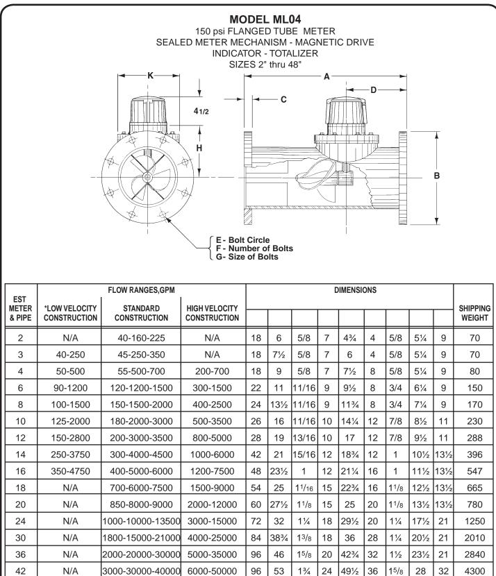
Standard construction will be supplied for all main line meters unless special flow range, materials, or construction are required. \* Low velocity (LV) construction has the same low and maximum flow rates as AWWA C704.
