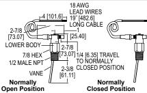
The **SERIES V10** Flotect<sup>®</sup> Mini-Size Flow Switches is designed to provide inexpensive. reliable monitoring of the presence or absence of flow in a system. This series is available for field installation in pipelines from 1/2 to 2" diameter and available in brass or 303 SS body.
