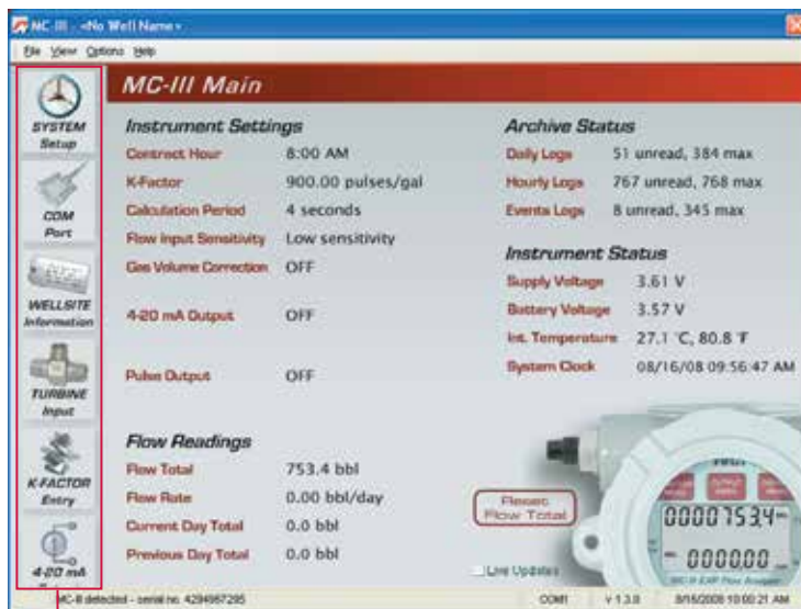
Users can access every configuration parameter from one screen.
