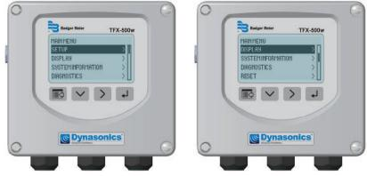
The cursor bar highlights the submenu or parameter that will be viewed or edited. The scroll bar on the right indicates the relative position the cursor bar is at on the list when there are more than 4 items.
