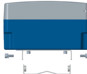
Figure 8: Secure the bracket
