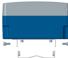
Figure 16: Secure the bracket
