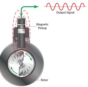
*Figure 1: B142 turbine flow meter*
